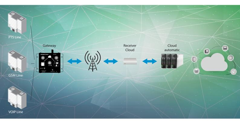
**SODI COM** is the remote connection solution for your lift to improve its continuous availability. Prevention and alert tool for maintenance, providing management and visibility for the owner or the plant pool manager, information for the user, **SODI COM connects all players involved with the lift.**
